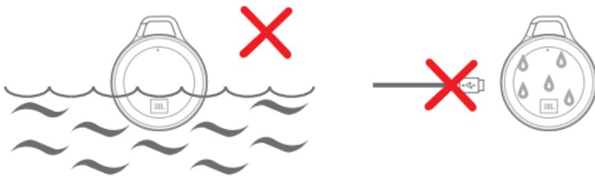
JBL Clip+ is splashproof; submerging it in water or other liquids may result in permanent damage to the speaker.
